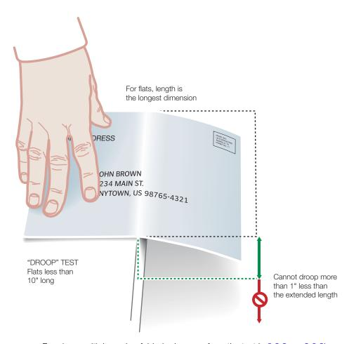
c. For pieces with bound or folded edges, perform the test in 3.2.3a or 3.2.3b above by placing the bound or final folded edge perpendicular to the edge of the flat surface.
