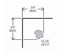
g. Continuous glue lines may be used as cover-to-cover seals for specific designs. When using glue as a sealing method, it must be placed along the entire length of the open edge and end no more than 3/4-inch from the open ends (see Exhibit 3.11g) unless standards require use of a continuous 1/2-inch wide glue line under 3.11h.
