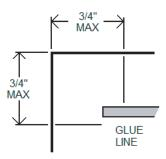
h. Continuous, 1/2-inch wide, glue lines must be placed along the entire length of the open edge and end within 1/16-inch of the open ends. The selvage along the open edge must not exceed 1/16 inch. Glue lines must be created with a permanent adhesive that is not tacky when dry.
