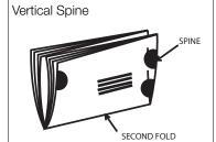
Cover paper weight—40-pound paper Two 1.5" nonperforated tabs on leading edge and one tab on trailing edge. Position upper tabs within 1-inch from the top edge. Position lower leading tab 0.5 inch from the bottom edge.
