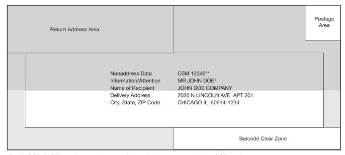
1.For MLOCR *FASTforward* users, the name of the recipient must appear in the OCR read area. Dark shaded area indicates "free space" for nonaddress printing. Light shaded area indicates preferred clear zone to enhance readability.
